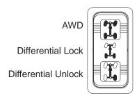
**Tip:** The AWD switch may be turned on or off while the vehicle is moving.
